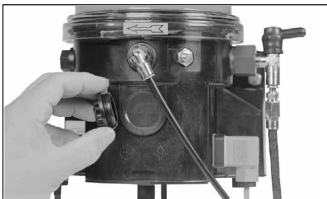
PCB 4 Cover lid to the control PCB
